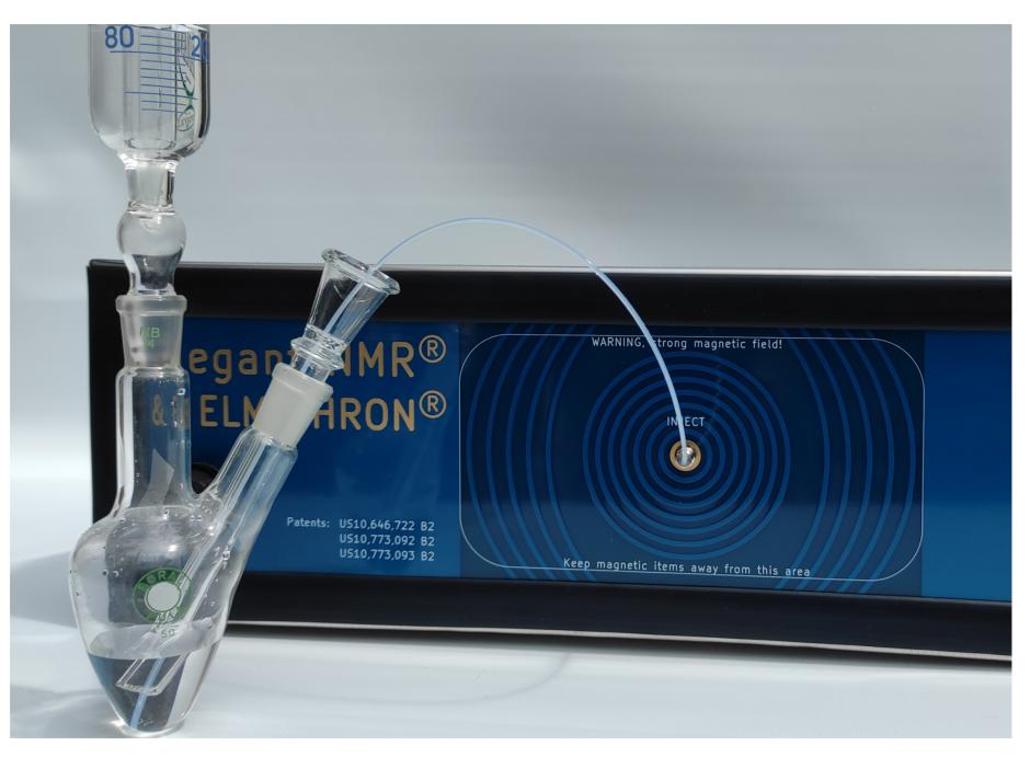
You must turn on Elmathron, connect a vacuum, start up the device, connect a capillary to the inlet and place the inlet capillary in the liquid to be measured.
